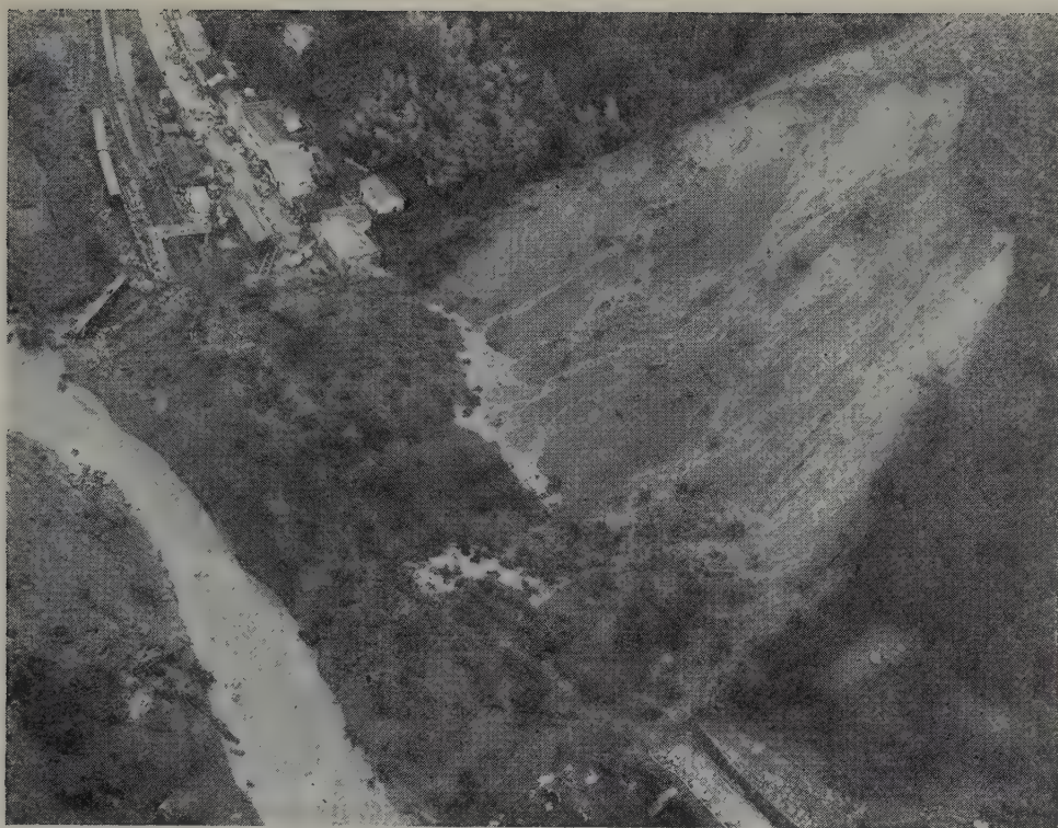
Fig. 2-6. The Shigeto railway station in Japan was partly buried by a landslide in 1972. The locomotive and two carriages were thrust into the river Ananai. The slope failure was triggered by torrential rain amounting to 742 mm per day (courtesy of Asahi Shinbun).
