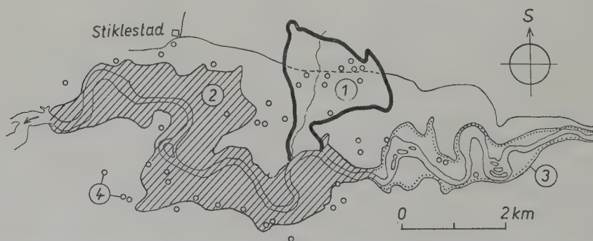
Fig. 1-3. Sketch map of the large landslip in Vaerdalen in 1893 (Holmsen 1953 ; 1 — head-scarp area, 2 — Vaerdalselven river-valley filled with liquid clay, 3 — temporary lake created by the damming of the valley, 4 — farms.
