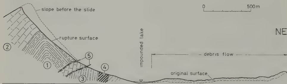
Fig. 1-5. Rockslide on Turtle Mountain in Canada, which destroyed part of the town of Frank; 1 — shaly limestone, 2 — solid limestone and dolomite (Carboniferous), 3 — sandstone and shale (Jurassic), 4 — Cretaceous sandstone and shale with coal seams, 5 — faults, disturbed zone (Cruden et al. 1978).
