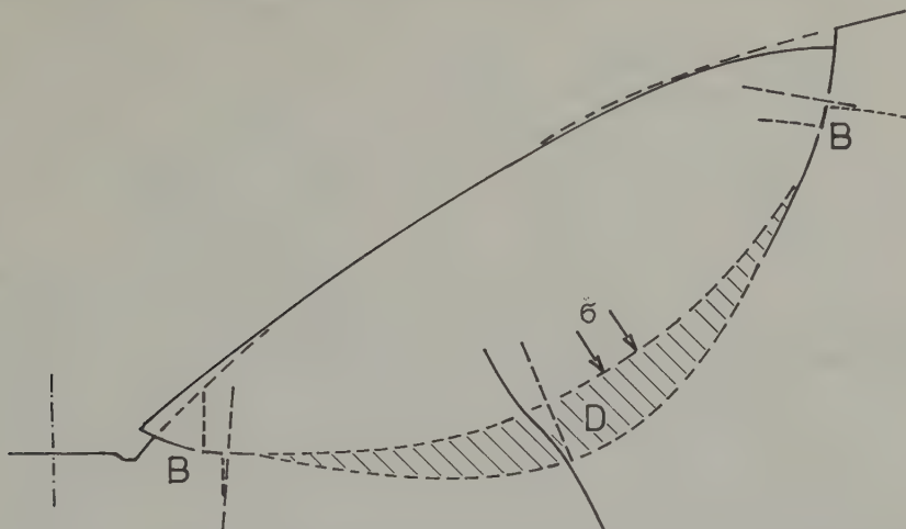
Fig. 4–8. Development of brittle shear failure B (a thin slip surface) and ductile shear failure D (a thick shear zone) in a slope (Menc 1968).
