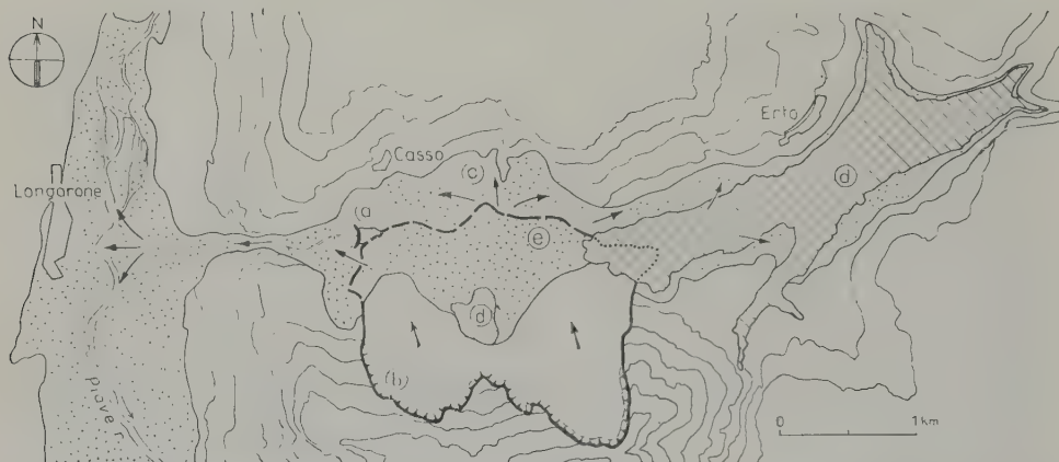
Fig. 10-14. Map of the Vaiont rockslide in the Italian Alps; a — dam, b — outline of the head area, c — area devastated by the high wave of water and by air pressure, d — lakes, e — outline of the slide body (after Selli and Trevisan, 1964).
